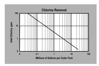
The graph above shows throughput capacity for chlorine removal using 2 gpm/cu.ft. of deionized water at 77°F with 0.1 ppm chlorine leakage endpoint.
