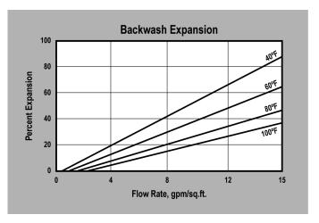
**BACKWASH** — The carbon bed should be backwashed at least once per week with chlorinated water to expand the bed 15 to 20 percent. This helps keep the carbon bed sterile and removes any foreign matter and carbon fines.
