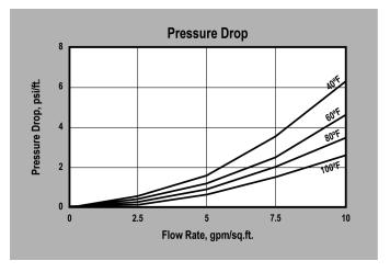
**PRESSURE DROP** — The graph above shows the expected pressure loss per foot of bed depth as a function of flow rate at various temperatures.
